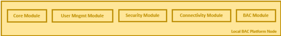
Figure 4.3.1: A platform node for BAC capabilities to be deployed in the building’s local datacentre.
