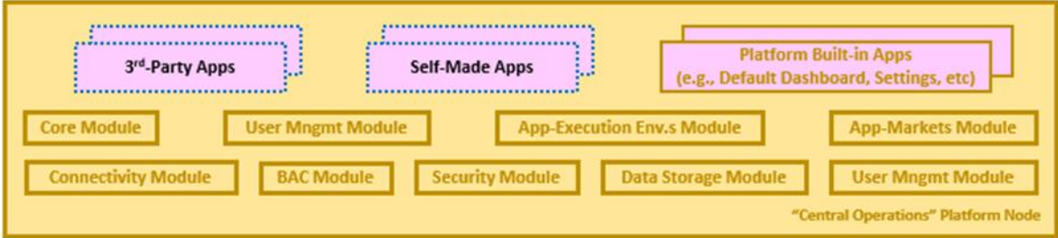
Figure 4.3.3: Indicative modules corresponding to a central operations platform node deployed on a cloud infrastructure.
