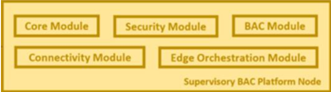
Figure 4.3.2: Indicative modules corresponding to a supervisory BAC platform node deployed to an edge datacentre.
